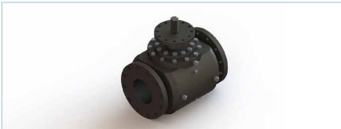
Top entry, cast steel, full bore ASME Class 150
